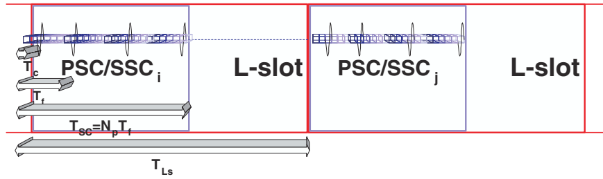
Figure 3.2: L-frame made up of M juxtaposed L-slots of length T_{L_s} . The SSCs are superimposed to a unique PSC.
