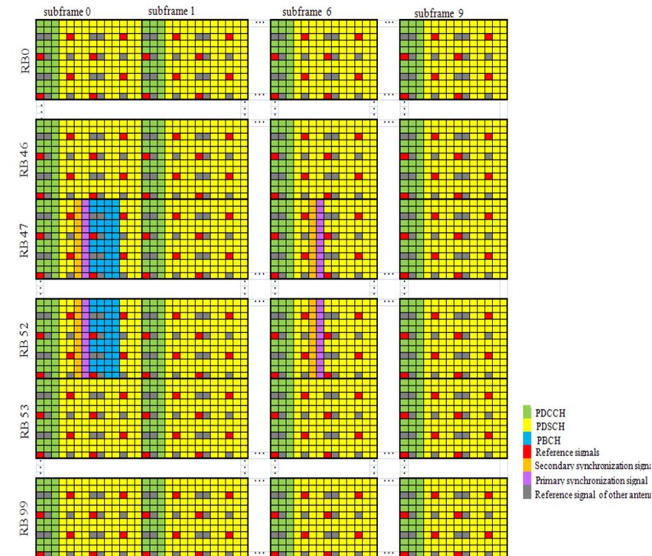
Fig. 4.22: LTE Downlink Channels 20 MHz 4 antenne
