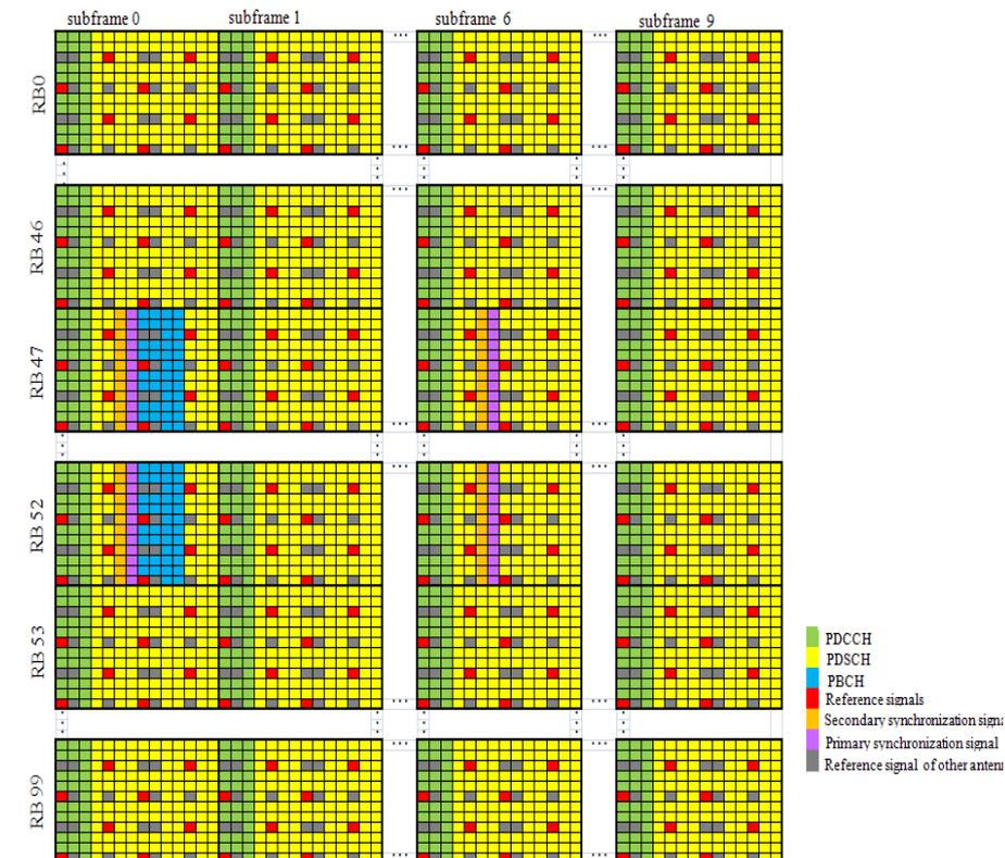
Fig. 1.4: LTE Downlink Channels 20 MHz 4 antennae
