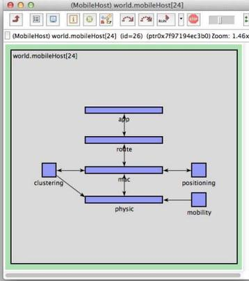
Fig. 2. Secondary node architecture implemented in OMNeT++.
