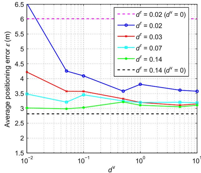
f0015 **FIG. 2** Average positioning error  $\bar{\epsilon}(d^r, d^v)$  for virtual fingerprinting, as a function of virtual RPs density  $d^v$ , and four different values of real RPs density  $d^r$ ; upper and lower bounds of the error are also shown, for real RPs only fingerprinting with  $d^r = 0.02$  and  $d^r = 0.14$ .
