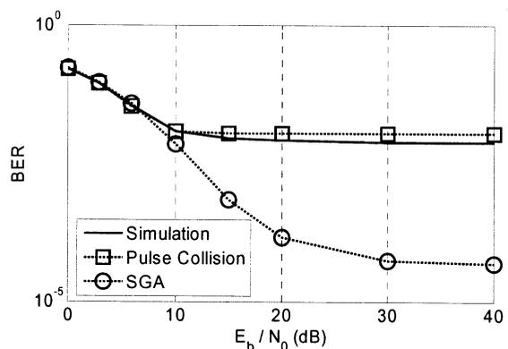
Figure 3 – BER vs.  $E_b/N_0$  with  $N_s = 1$ ,  $T_s = 60$  ns,  $N_i = 5$ ,  $E^{(1)} = E_u$ ,  $E^{(2)} = 4E_u$ ,  $E^{(3)} = 8E_u$ ,  $E^{(4)} = 1/4(E_u)$ , and  $E^{(5)} = 1/8(E_u)$ .
