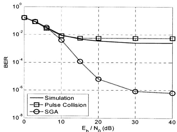
Figure 2 – BER vs.  $E_b/N_0$  with  $N_s = 1$ ,  $T_s = 60$  ns,  $N_i = 3$ ,  $E^{(1)} = E_u$ ,  $E^{(2)} = 4E_u$ ,  $E^{(3)} = (1/4)E_u$ .
