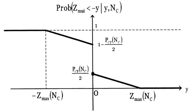
Figure 1 – Linear model for the conditional probability of error  $\text{Prob}(Z_{\text{mui}} < -y | y, N_c)$ , given  $y$  and given  $N_c$ .
