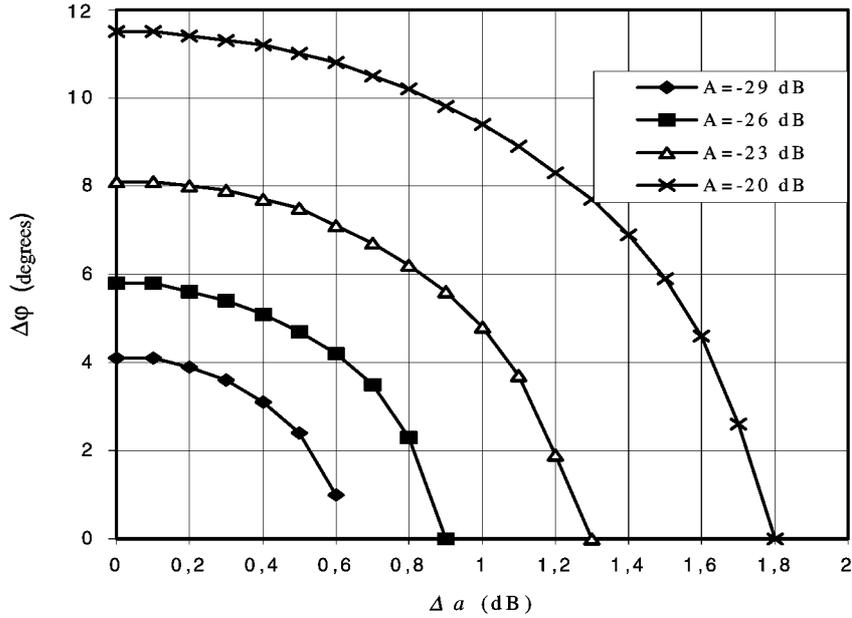
Figure 5. Locus of the points, in the plane  $\{\Delta a_{\text{dB}}, \Delta \varphi_{\text{degree}}\}$  for which  $20 \log_{10} a < A_{\text{dB}}$ .
