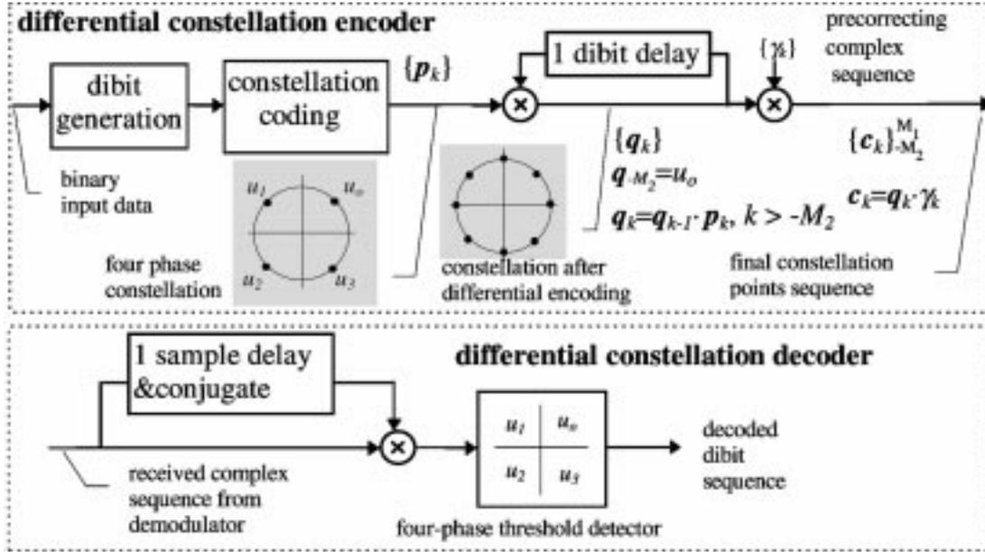
Figure 3. Block diagram of the differential co/decoder.
