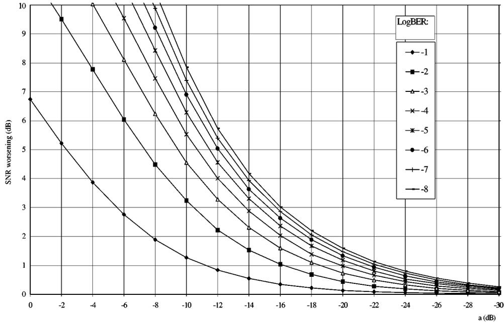
Figure 4. SNR degradation versus  $a$  (dB), for different values of  $\log_{10}(\text{Bit Error Probability})$  evaluated @  $a = 0$ .
