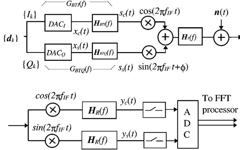
Figure 2. Block diagram of the baseband equivalent of the analog TX/RX connection.
