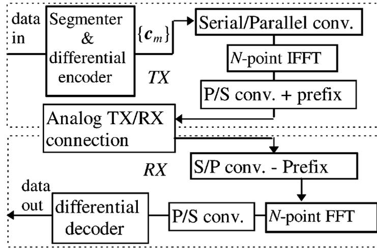
Figure 1. Block diagram of an OFDM modem.
