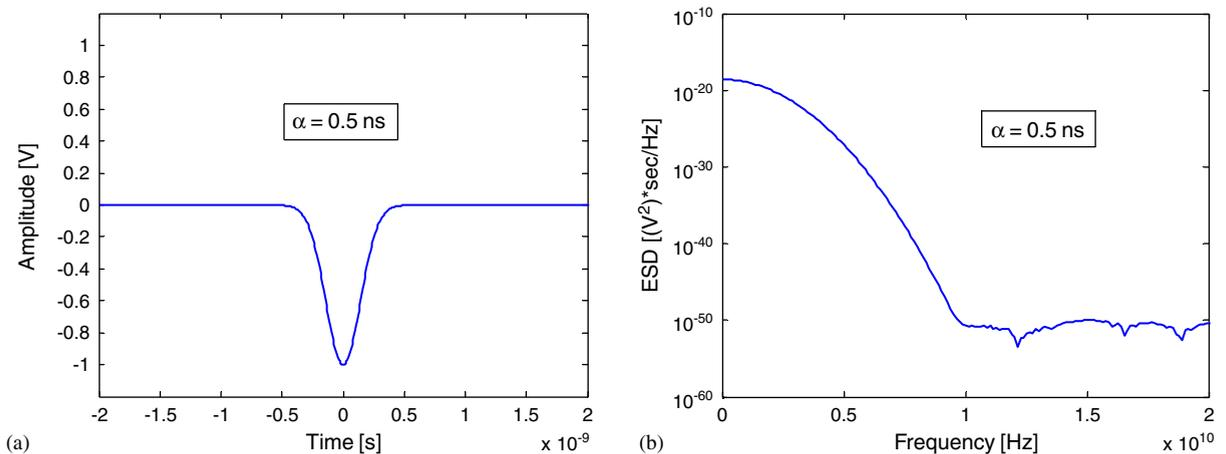
Fig. 1. Example of a Gaussian pulse: (left) voltage waveform, and (right) corresponding ESD.
