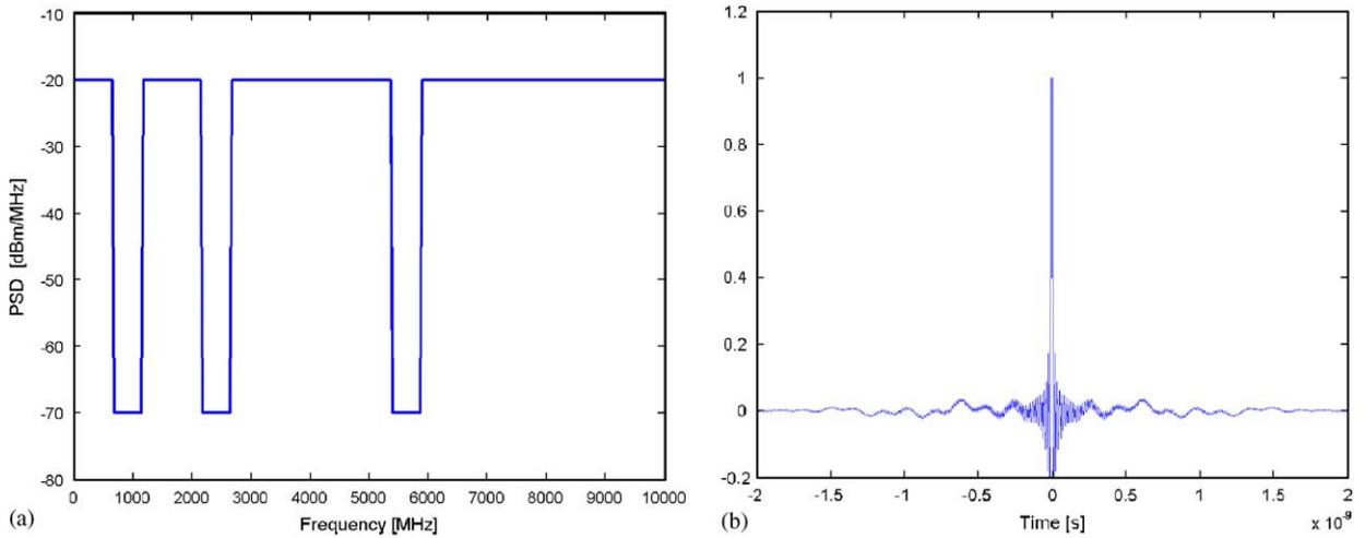
Fig. 4. Target radiated PSD for mitigation of the effects of narrowband interference in the ISM bands on a UWB receiver (a), and corresponding amplitude-normalized voltage waveform associated with the radiated PSD (b), that is the voltage of (b) has a radiated PSD as of (a).
