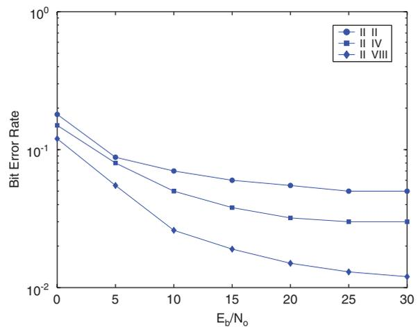
Fig. 6. BER vs.  $E_b/N_0$  for different adopted pulses in two UWB networks N1 and N2 (Circles: both N1 and N2 use the II Gaussian derivative; Squares: N1 and N2 use the II and IV Gaussian derivative, respectively; Diamonds: N1 and N2 use the II and VIII Gaussian derivative, respectively).
