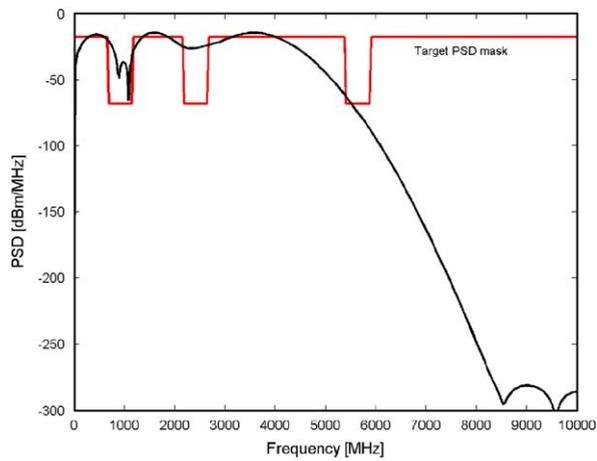
Fig. 5. PSD of the linear combination of Gaussian waveforms obtained by waveform matching with  $\alpha = 0.714$  ns for all derivatives vs. target PSD mask.
