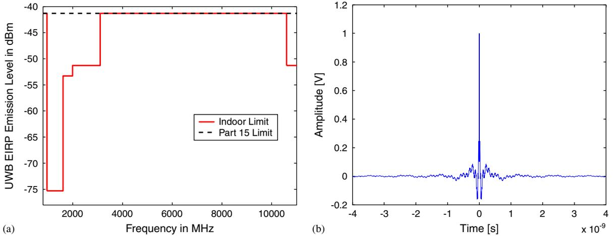
Fig. 2. FCC indoor emission mask for UWB devices [1] (a), and corresponding amplitude-normalized voltage waveform (b). The pulse of (b) satisfies Eq. (16) and has a radiated PSD as of (a).
