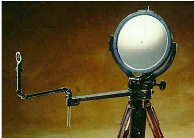
A British Mark V Mance pattern 5-inch heliograph.
