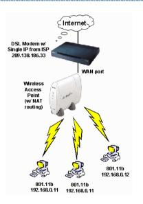
Access Control in these networks is typically demanded to the element connected to the fixed network, which coordinates the access of wireless devices by managing the resource available in the system for transmissions
