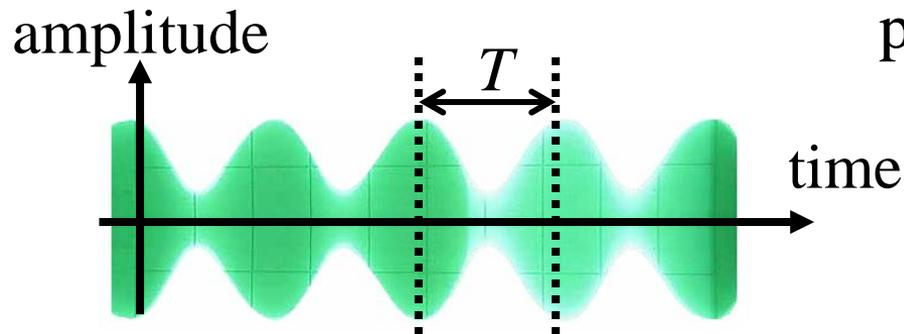
*Example of continuous-time, RF modulated digital signal with pulse rate  $1/T$*
