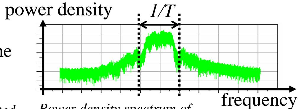
*Power density spectrum of the transmitted signal*
