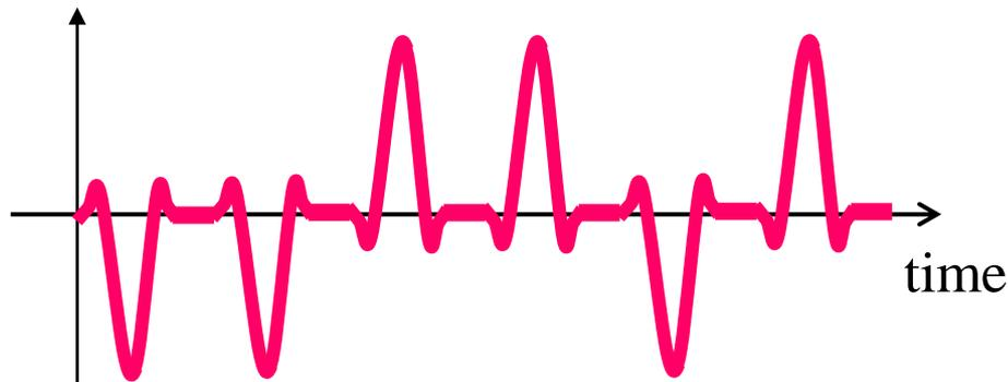
Signal at the output of the pulse shaper
