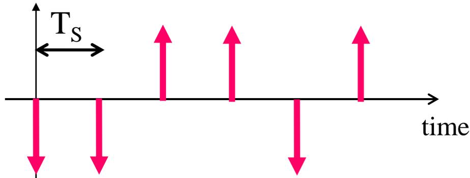
Signal at the input of the pulse shaper
